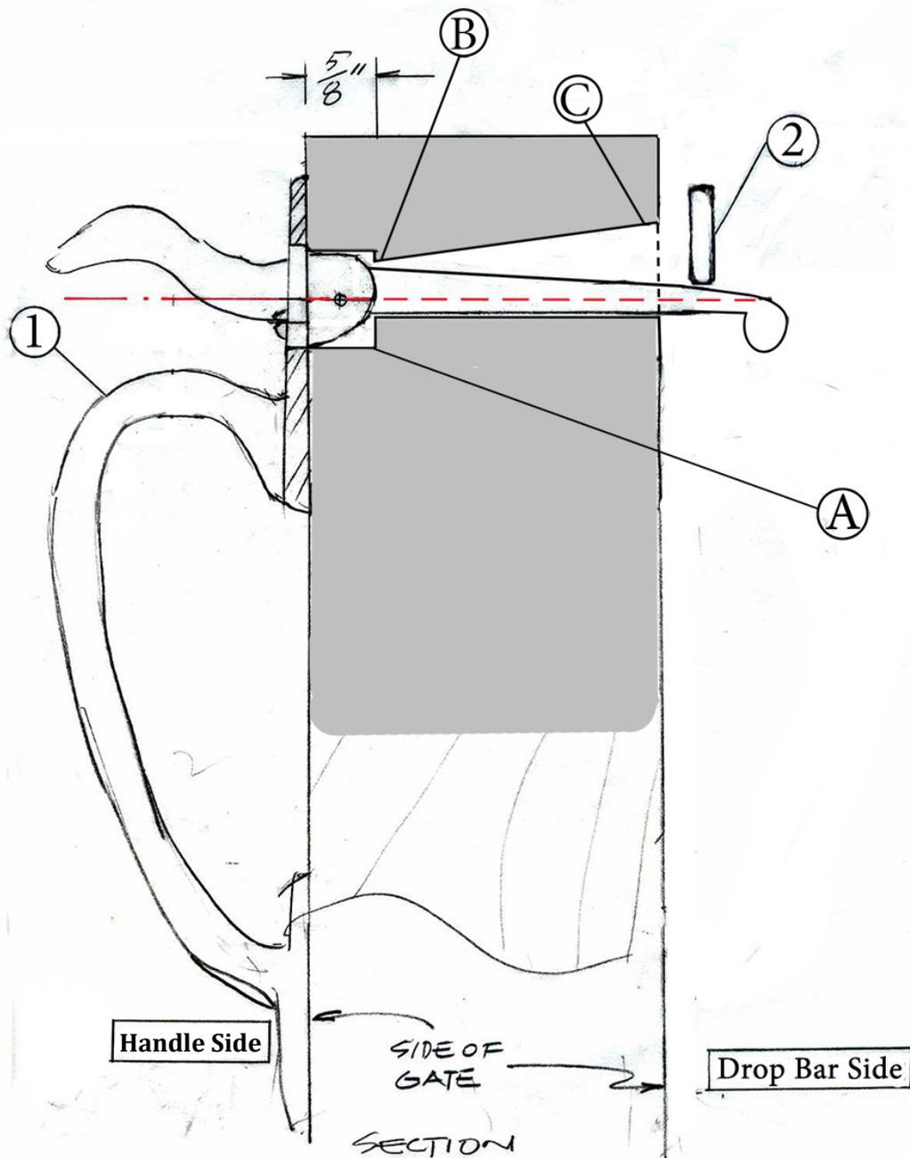
Gate should be hung on its hinges before installing latch hardware [but it may be easier to drill holes if it is removed and done on a work bench]. There should be between a  $\frac{1}{4}$ " and  $\frac{1}{8}$ " vertical clearance gap between the gate and its post or frame.
