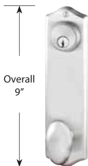
• Egg Knob with Keyed Colonial Plate • Two Standard 2 1/8" Door Preps • 5 1/2" Center to Center Hole Spacing
