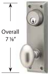
• Egg Knob with Keyed Quincy Plate • Two Standard 2 1/8" Door Preps • 3 3/8" Center to Center Hole Spacing
